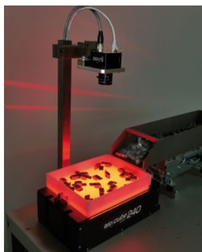
Fig. 2 Asycube feeders are very flexible and suitable for extremely gentle feeding of loose parts and components of all geometries with sizes from less than 0.1 mm up to 150 mm. (Source: Asyri)
