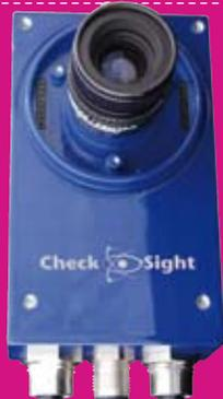
resolution, high-dynamic range, global shutter CMOS or progressive-scan CCD without smear effects."
